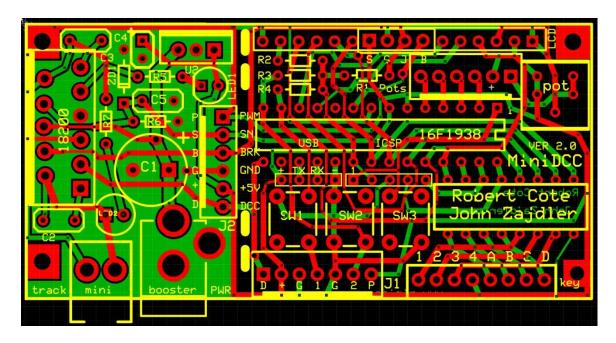
Preliminary PCB (soon to be available on the Web site) and Schematic for optional potentiometer control and imbedded USB/UART interface.
